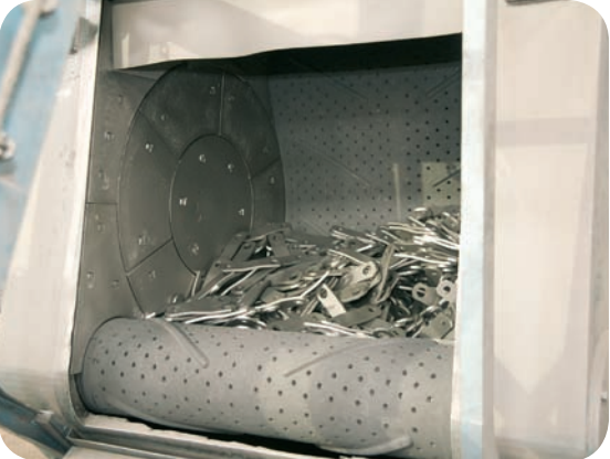
Shot peening parts improve fatigue and crack resistance
