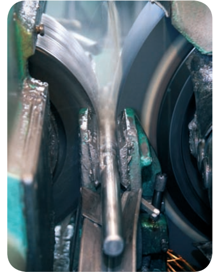
Pins are ground to thoroughly optimize the wear life.
