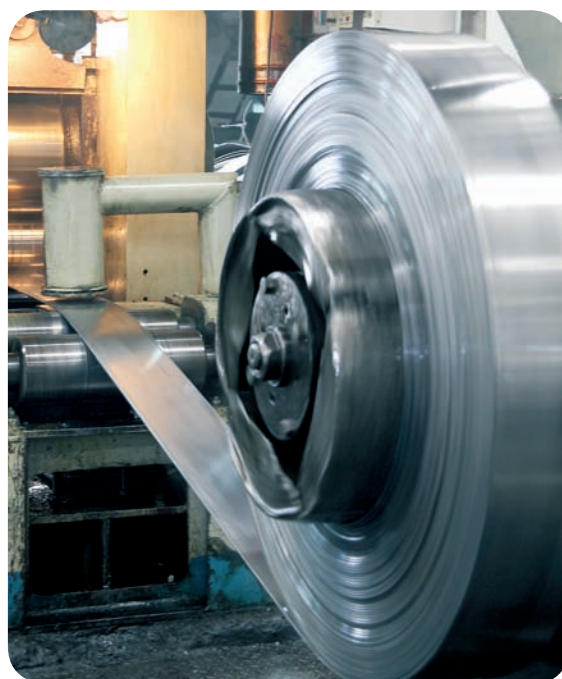
Continuous rolling machine to achieve uniform thickness of plate material
