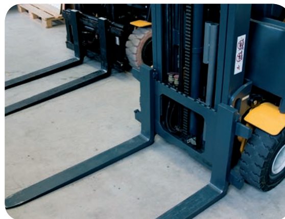
Leaf chain used for lifting in a forklift mast
