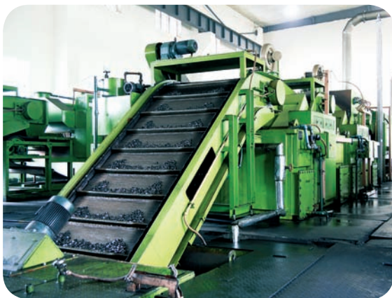
Conveyor furnace line used for roller and bushing heat treatment e.g. carbon-nitriding
