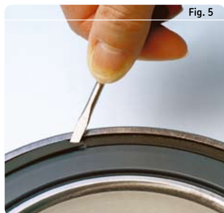
Removing a retaining ring
