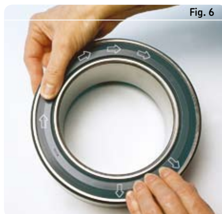
Inserting the seal in the outer ring
