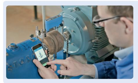
Shaft alignment is recommended for almost every industry, as it enables machine uptime to be significantly improved and maintenance costs to be reduced. The TKSA 11 focuses on industries where these shaft alignment benefits have not yet been realised and helps customers profit from correctly aligned shafts.
