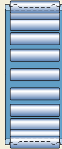
Machined steel cage of the radial bearing
