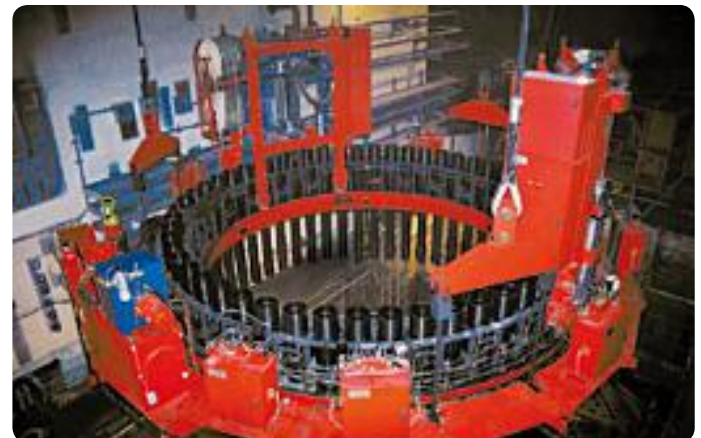
Automatic MST Machine holding 54 vessel studs lowering down to the reactor vessel for closing operation
