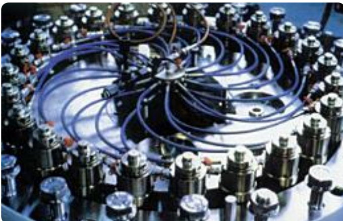
Central feed individual tensioner simultaneous tightening
