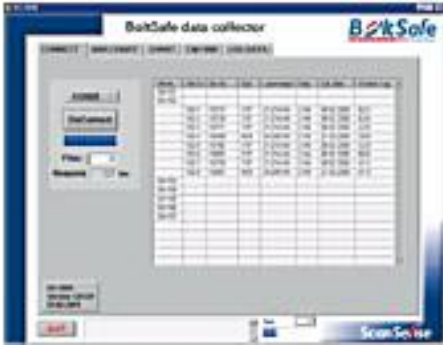
The BS-2000 software processes the data from the BoltSafe washers
