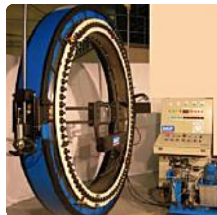
Machine to tighten simultaneously the fastening bolts of the blade slewing bearings on wind turbine
