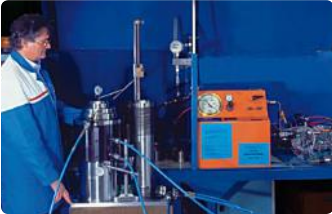
Hydraulic test beds (using oil and water), for low-pressure tests (0-300 bar), and high pressure tests (300-3 000 bar)
