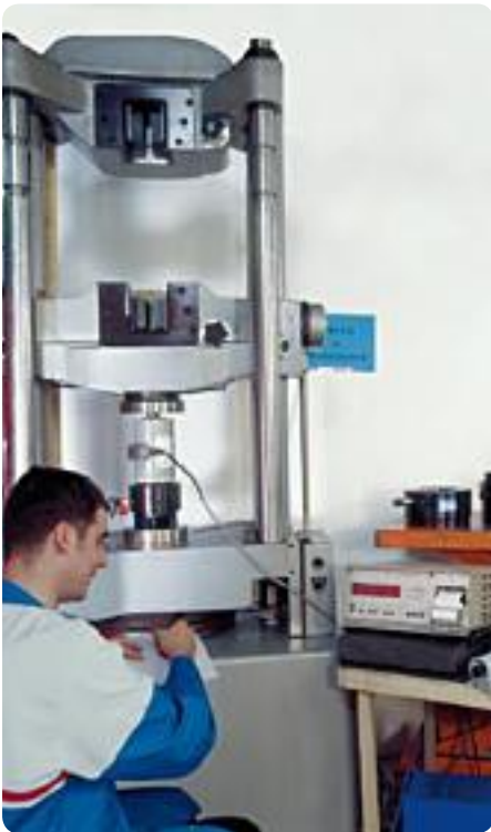
Mechanical test beds to measure loads, stresses and strains, to determine equipment performance and lifetime
