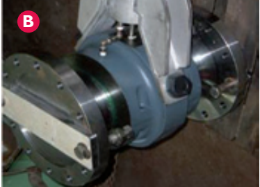
The custom-built Cooper solution in picture B combined a triple boss hanger mounting with split roller bearing equipped with double sealing and air purge provision on each end.
