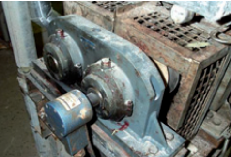
Picture A shows a plain bearing on a scroll conveyor at a French sugar plant where short bearing life, shaft wear and product contamination from oil and rust were causing major problems.
