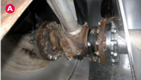
Picture A shows a plain bearing on a scroll conveyor at a French sugar plant where short bearing life, shaft wear and product contamination from oil and rust were causing major problems.
