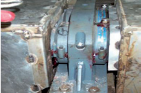
The custom-built Cooper solution in picture B combined a triple boss hanger mounting with split roller bearing equipped with double sealing and air purge provision on each end.
