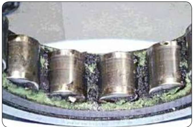
Lubricant degradation caused by electrical discharge currents.
