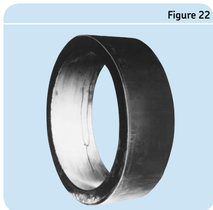
Cracks caused by faulty housing fit
