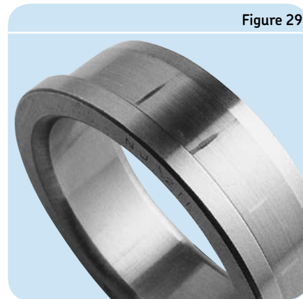
Smearing caused by excessive force in mounting
