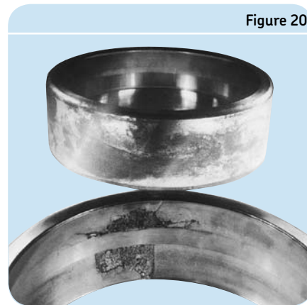
Advanced wear and cracking due to fretting corrosion
