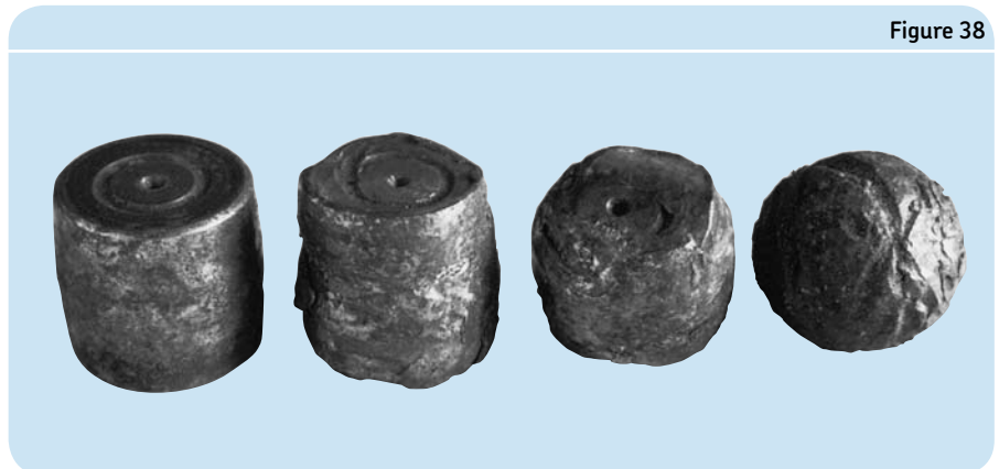
Discoloration and softening of metal caused by inadequate lubrication and excessive heat
