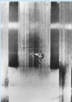
Early fatigue spalling
