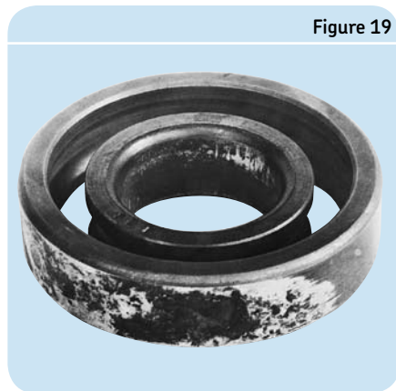
Wear due to fretting corrosion
