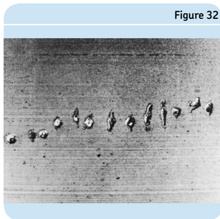
Electric pitting on surface of spherical outer raceway caused by passage of relatively large current
