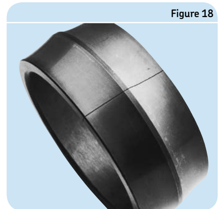
Axial cracks caused by an excessive interference fit
