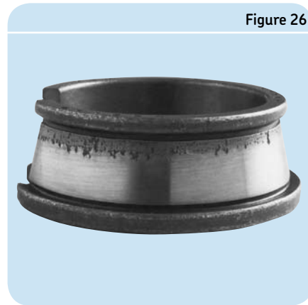
Fatigue caused by edge loading
