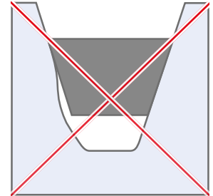
Worn out V-grooved pulley
