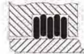
YSK Series QSK Series External - Medium Duty 1 set = 5 individual rings (3 rings rotate with shaft & 2 rings rotate with bore)
