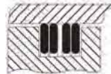
YHD Series QHD Series Internal - Medium/Heavy Duty 1 set = 2 individual rings (rings rotate with bore only)
