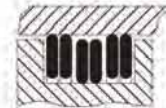
YHKD Series QHKD Series Internal - Heavy Duty 1 set = 3 individual rings (2 rings rotate with bore & 1 ring rotates with shaft)
